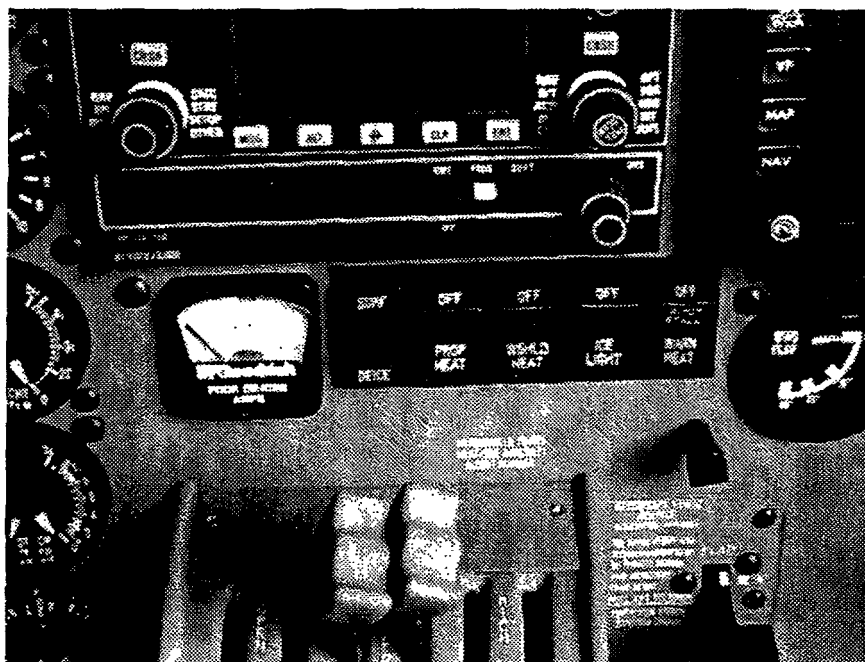
ICE DETECTION LIGHT, SURFACE DEICER, PROPELLER DEICER AND HEATED WINDSHIELD CONTROL SWITCHES
